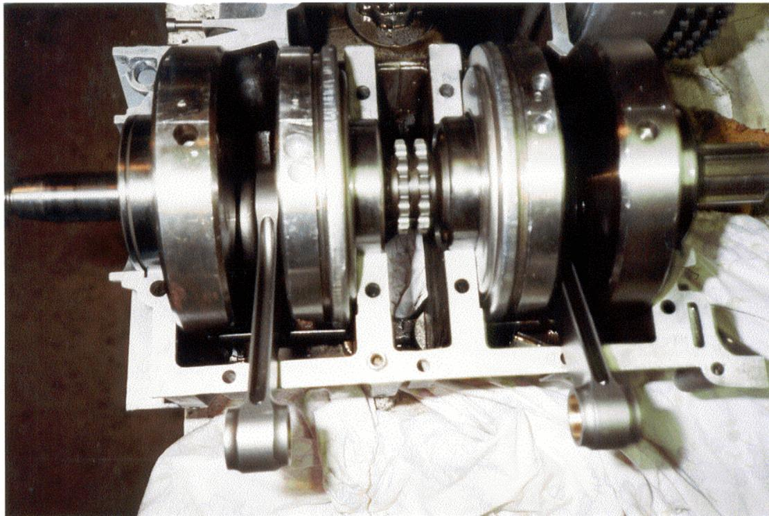
**Figure 2. My 750 SF2 crankshaft with holes drilled in the outer webs.**
